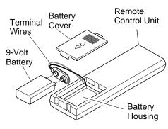
Figure 30 - Installing Battery in Hand-Held Remote Control Unit
